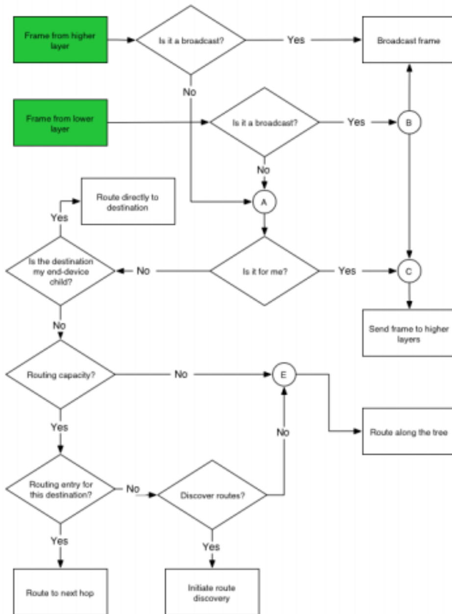
Figure 57 Basic routing algorithm
